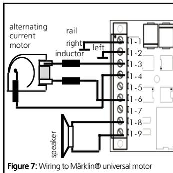
Figure 7: Wiring to Märklin® universal motor
