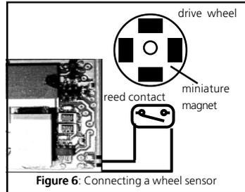
Figure 6: Connecting a wheel sensor
