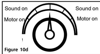
Operation using a conventional DC controller is possible without any problems except for one limitation. The engine will only start moving when the track voltage reaches 7–8 Volts. Maximum speed will be reached when turning the controller to the limit. This is absolutely normal and is due to the minimum voltage the LokSound decoder requires for operation. Running sounds are available in this operating mode but not additional sound effects.
