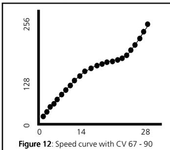
Figure 12: Speed curve with CV 67 - 90
