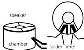
LokSound decoders may only be used with the speakers supplied by ESU GmbH & Co. KG. They have an impedance of 100 Ohm. The use of speakers from other manufacturers may cause considerable distortion and in extreme cases, may even destroy the LokSound decoder.
